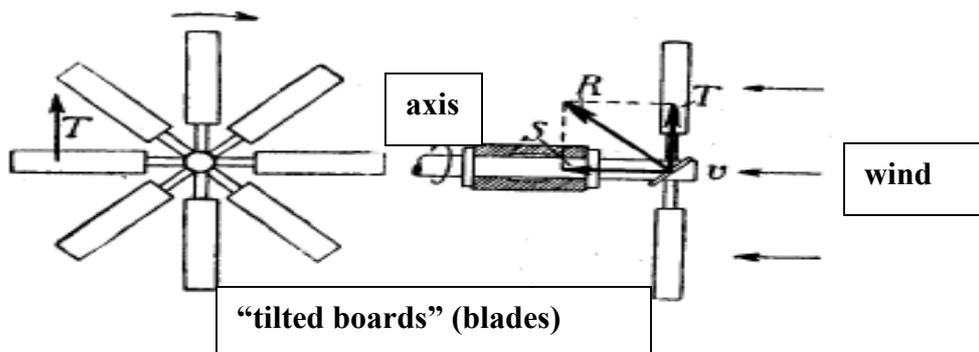
By the way, a fan that cools us with air during hot weather is also a windmill, but an "inverted" one. Instead of generating electricity with wind it generates wind with electricity. If we connect the motor of the to the current, the motor will make rotate the blades and they will produce the air we feel in the face. If we turn the fan 90 degrees, in principle we could use it to generate energy.
