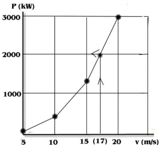
If for example we want to know the power of the windmill in our example at a wind speed of 17 m/s, instead of calculating this power with the formula we just have to find the point on the curve corresponding to this wind speed (17 m/s) → about 2000 kW (follow the arrows).
